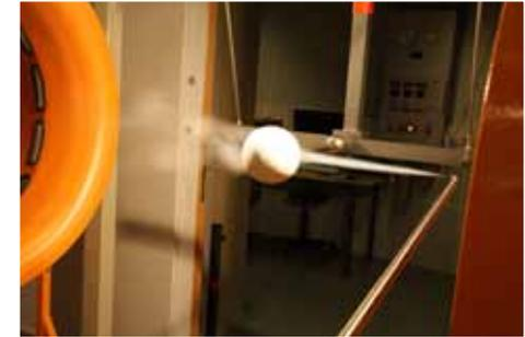
We also offer the FlowLiner® – our **special device** for generation fog even at **high air velocities**. The FlowLiner® enables you to examine air flow conditions at air velocities of more than 2 m/sec, e.g. in a wind tunnel.
